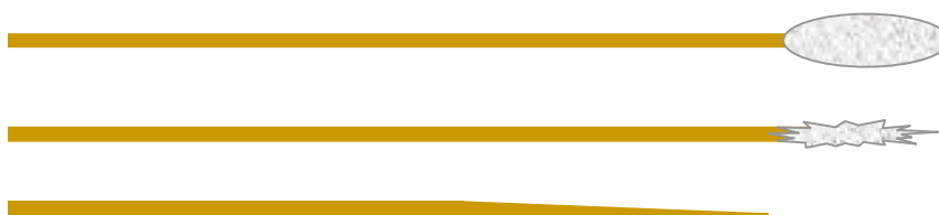
Figure 5. Cotton swabs on wood sticks are useful cleaning tools for MAS rotors and caps.
