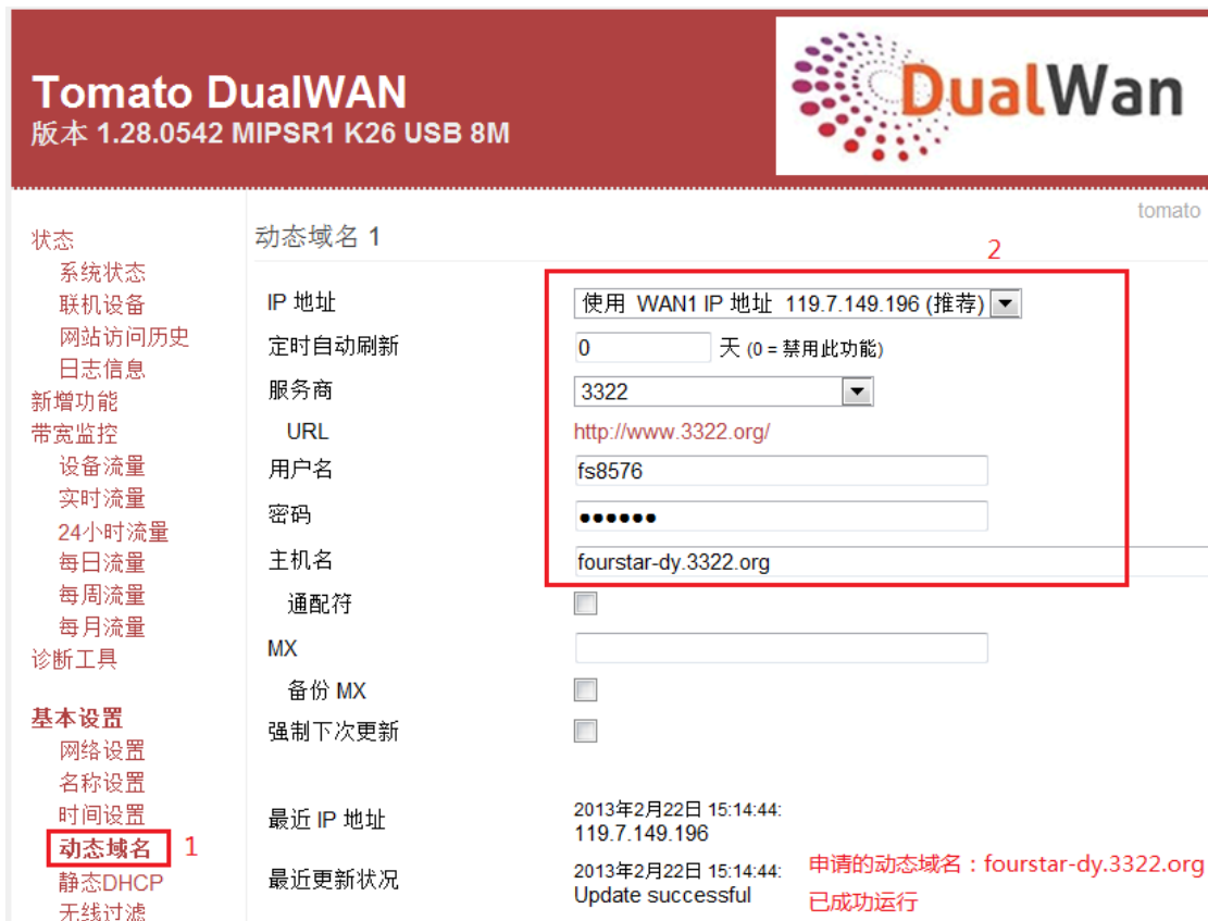
Figure 6-3 setting dynamic domain name on the router
