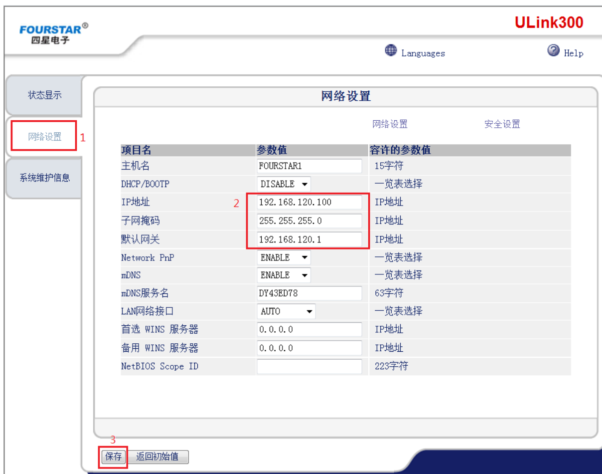
Figure 6-5 Setting ULink300 IP address and other parameters
