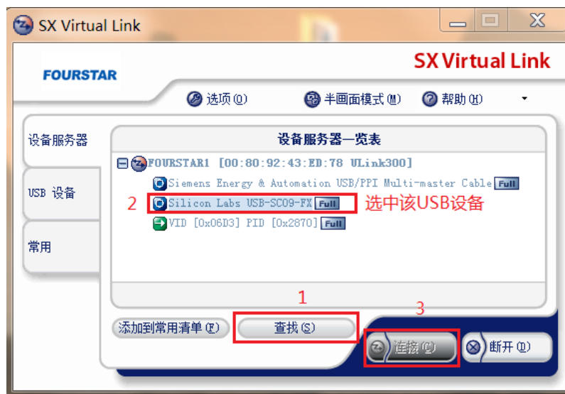
Figure 6-11 connecting USB equipment
