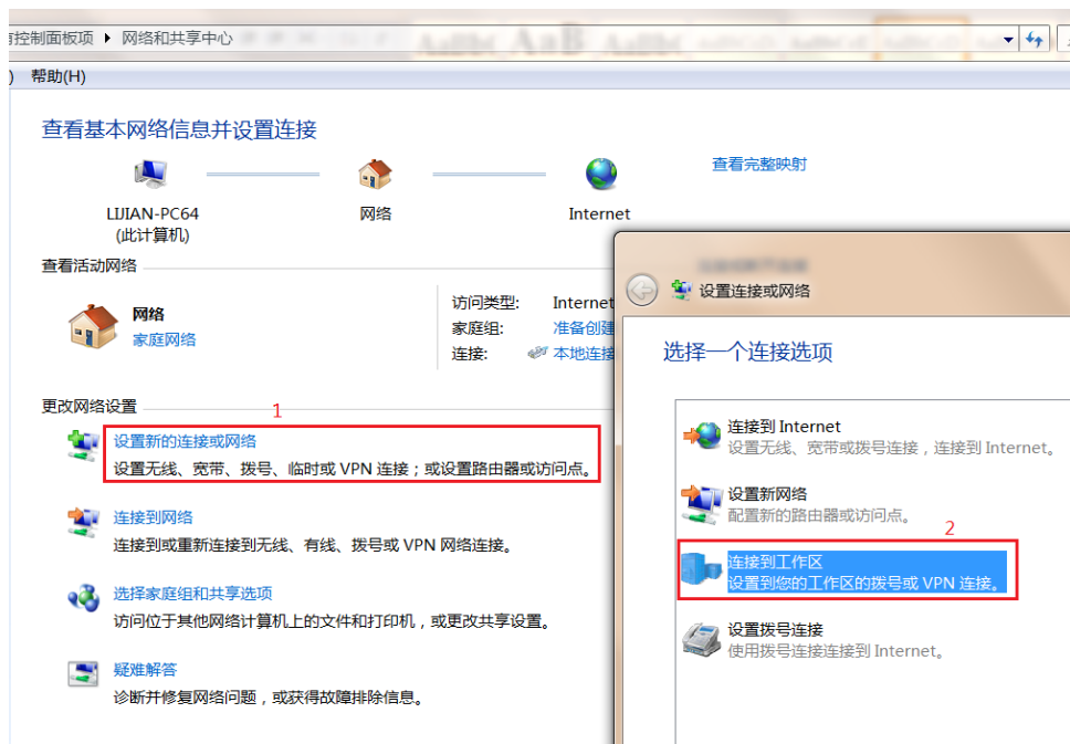
Figure 6-6 Setting VPN connection
