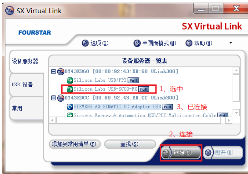
Figure 5-5 interface of SX Virtual Link connection software
