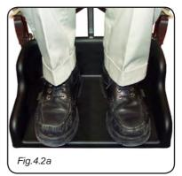
• If the BB has been set up to use an integral footrest (Fig.4.2a), then the wheelchair footrests are not to be used.
