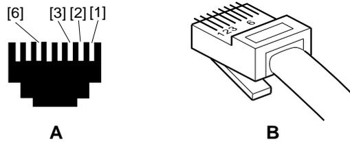
Figure 1: Pin assignment of an RJ45 plug connector
