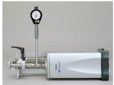
Using the interchangeable anvil clamp (part of Bore Gage Accessories, 02ASK110) (Applicable to Mitutoyo's bore gages only.)
