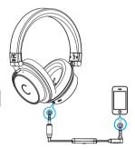
Audio jack configuration on airplanes vary. For a single 3.5mm jack, use the single plug. No adaptor needed. To connect to dual output connectors, use the supplied dual 3.5mm plug adaptor
