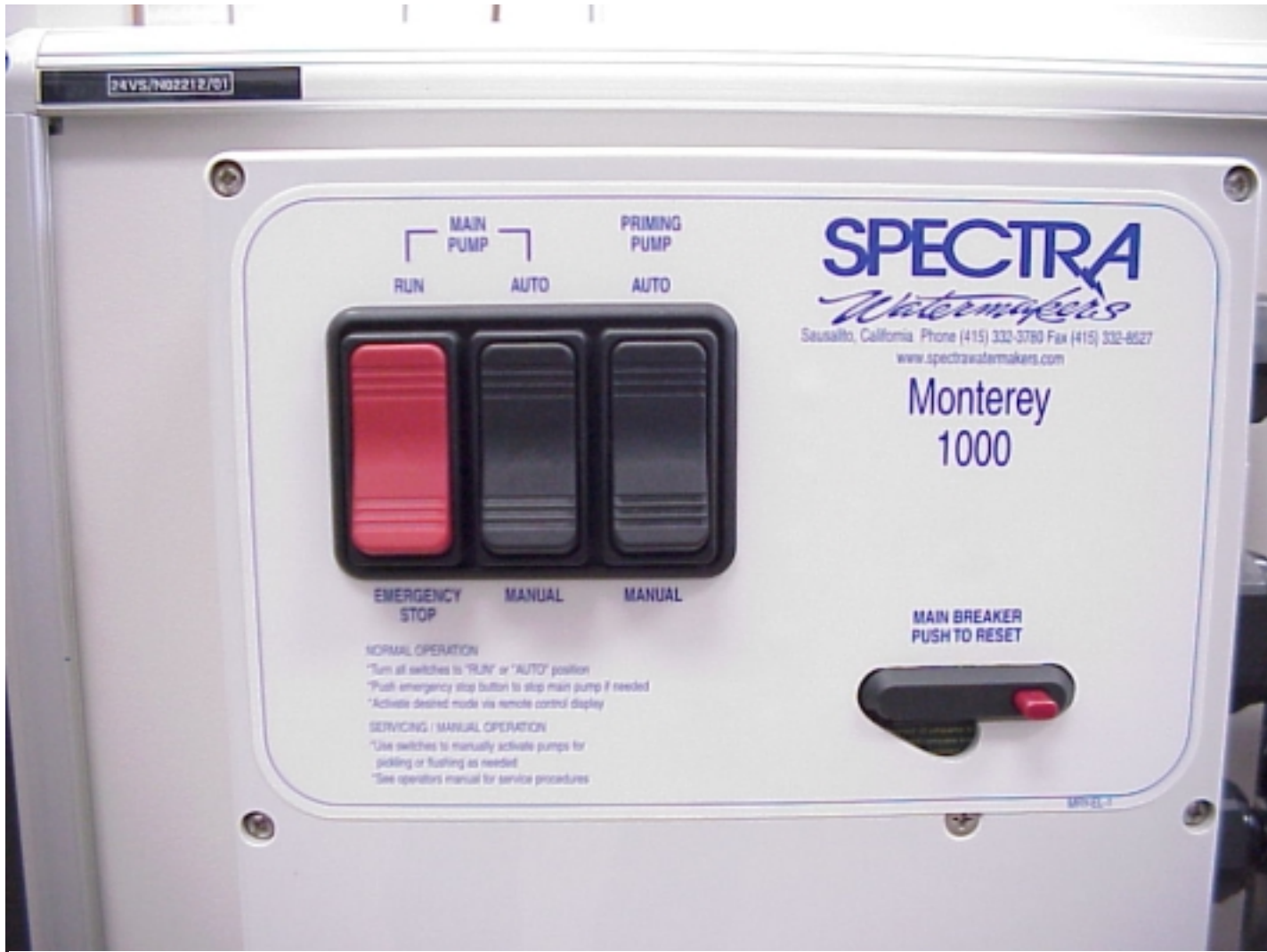
Monterey DC Main Breaker, Emergency Stop & Manual Control Switches
