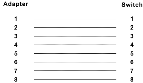
Fig. 3-12 Pin assignments for straight-through cabling
