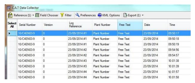
To change the job reference field, for example to highlight a particular survey with a reference ID, select the row(s) with the mouse and click reference. Input the Log reference, Plant Number or enter Free Text and this will now appear in the relevant columns:
