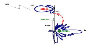
Isolation becomes particularly problematic when Omni-directional antennas are used for both the Donor and the Coverage antennas. Since these antennas transmit in a circle (or more accurately a sphere) it is very easy for these spheres to overlap and thus negate the repeater system.
