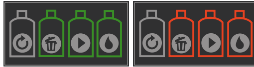
Figure 4.6: Fluid container status symbols. Left: Fluid containers are ready. Right: Fluid containers need replaced.
