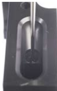
Figure 12.5: Test calibration of the needle arm position in the washing station. The position of the uptake needle should appear as shown above.
