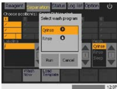
Figure 6.21: "Wash Now" command displays two options: "Qrinse" (quick rinse) and "Rinse". A full rinse is required for instrument priming.
