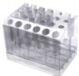
Figure 12.8: Bottom detection calibration. In the case of a Chill 5 Tube Rack the needle will be positioned midpoint (equidistant) to tube coordinates A1, A2, B1, B2.
