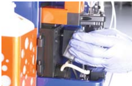
Figure 12.20: Inserting the 2D code reader.
