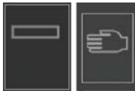
Figure 4.12: MACS MiniSampler status graphic. Left: The MiniSampler was successfully installed. Right: No MiniSampler was detected.
