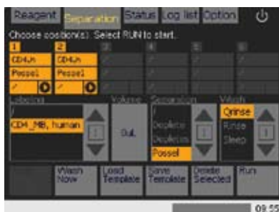
Figure 6.23: The current display indicates that autolabeling will be performed on both samples.
