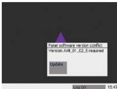
Figure 12.2: The user must confirm any update. The current software (panel software version) will be overwritten.
