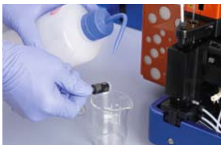
Figure 7.8: Washing the pump syringe with distilled water.
