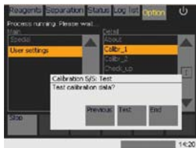
Figure 12.12: It is important to test the new calibration settings. To navigate back through the calibration steps, select “Previous”.
