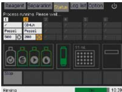
Figure 6.28: Monitoring the status during cell separation. Sample processing at position 1 is completed (white color). Sample at position 2 has finished the separation and is now performing a Rinse.
