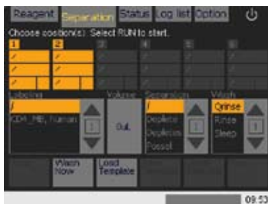
Figure 6.22: Sample positions 1 and 2 were selected. The purpose of this example is to demonstrate how sample processing conditions can be easily modified and to clarify the differences between autolabeling and manual labeling. Alternatively, each sample could be programmed individually.
