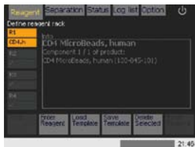
Figure 6.4: CD4 MicroBeads, human (# 130-045-101) was identified by the 2D code reader software and assigned to the reagent rack position “R1”.
