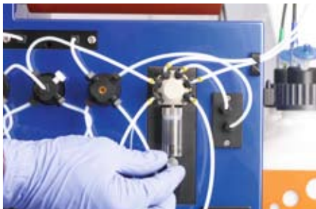
Figure 7.5: Unscrewing the plunger lock screw.
