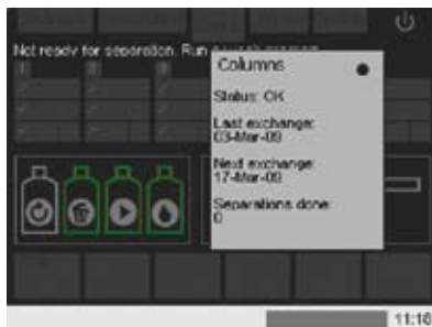
Figure 4.9: Column status. By touching the column symbol a pop-up box displays a text report of the column status.
