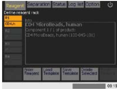
Figure 6.15: CD4 MicroBeads, human vial was placed onto the MACS Reagent Rack position "R1".
