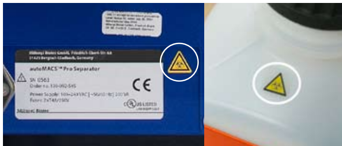
Figure 1.4 Warning signs for biohazard located on lower facing panel of the autoMACS Pro Separator (left) and top of autoMACS Pro Separator fluid bottle (right).
