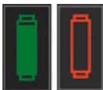
Figure 4.8: The column status graphic. Left: The column is ready. Right: The column must be changed.
