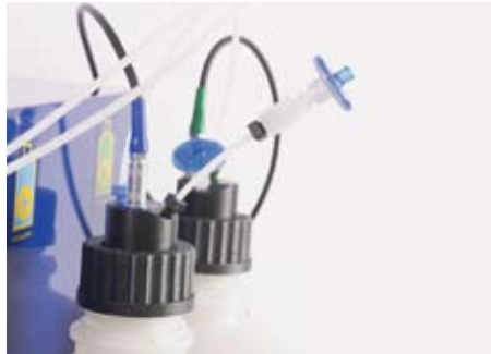
Figure 7.24: Hydrophobic air filter attached to a fluid container.
