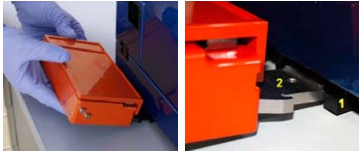
Figure 3.4: Location of the MiniSampler guide (2) and receiving slot (1) for the MACS MiniSampler.
