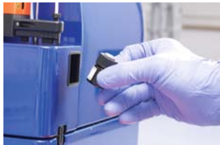
Figure 6.3: Scanning a reagent vial using the 2D code reader. In this example, the vial “CD4 Microbeads, human” was scanned.
