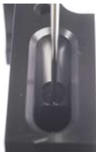
Figure 3.16: Test calibration of the needle arm position in the washing station.
