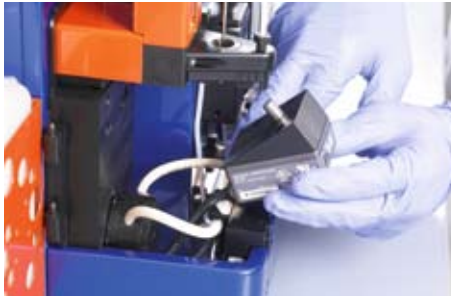
Figure 12.19: Make sure that 2D code reader cable is located in between the peristaltic pump tubes.
