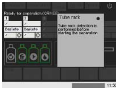
Figure 4.11: Tube rack status text box: No rack is detected until cell separation is performed.
