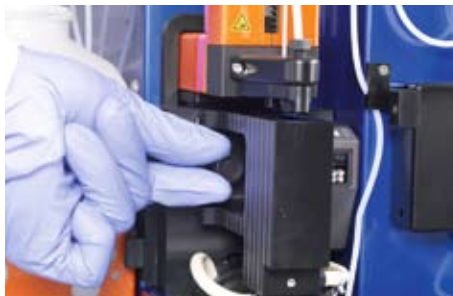
Figure 7.11: Unscrew the thumb screw.
