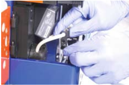
Figure 7.22: The waste distributor.
