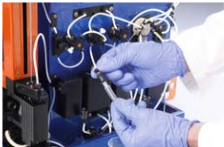
Figure 3.22: Unscrewing the top column connector for column removal.
