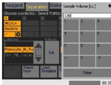
Figure 4.16: Entering the sample volume in microliters ( \mu\text{L} ) for Monocyte Isolation Kit II, human.
