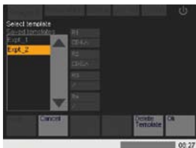
Figure 6.13: Selecting a reagent template. Expt_2 was selected which comprises of CD4.h and CD8.m on positions R1 and R2, respectively.
