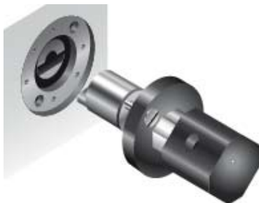
Figure 7.17: Inserting the new valve.
