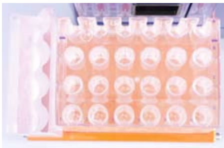
Figure 3.12: Positioning the Chill Rack 5 adjacent to a MACS Reagent Rack 4 on the MACS MiniSampler.
