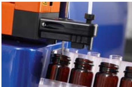
Figure 3.18: Test calibration: Control position of needle in vial.
