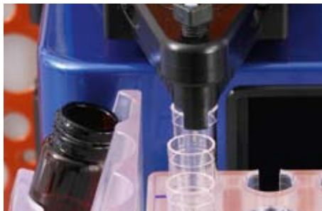
Figure 12.10: The uptake needle should be positioned as shown above.
