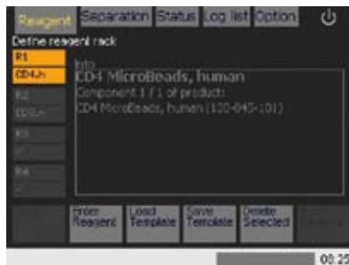
Figure 6.11: Using the 2D code reader, two reagent vials were assigned to the reagent rack positions “R1” and “R2”.
