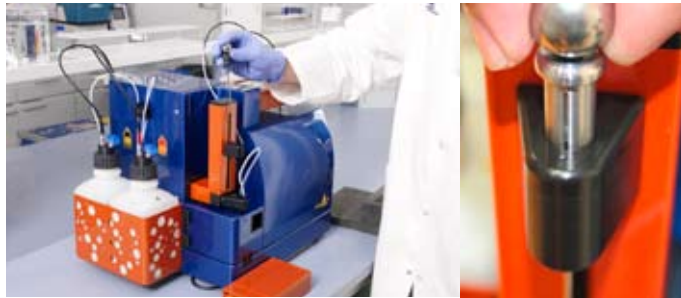
Figure 3.9: The needle port is positioned as illustrated above.
