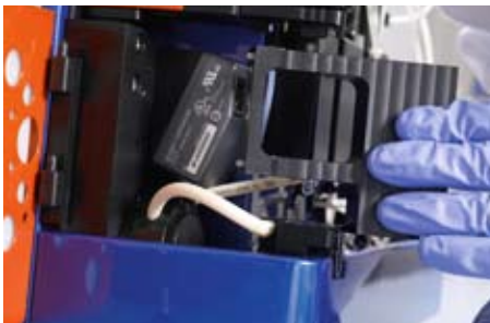
Figure 12.22: Reinstall washing station.
