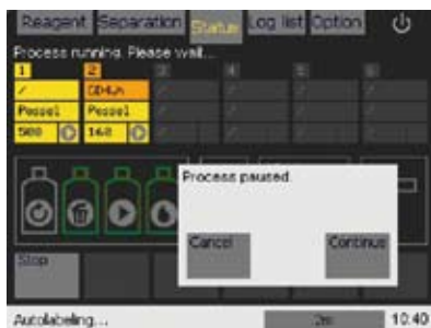
Figure 6.29: Select “Stop” to pause cell separation. To continue cell separation select “Continue”. To cancel the entire procedure, select “Cancel”.
