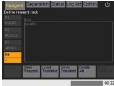
Figure 6.10: To delete all reagents from the reagent rack, an unassigned position on the reagent rack must be highlighted. In this example the only unassigned position “R4” was selected.
