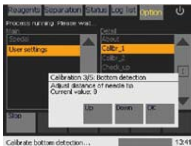
Figure 12.9: If necessary, adjust the z-axis of the needle tip using “Up” and “Down” navigation tools.
