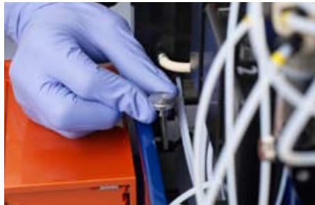
Figure 3.5: Securing the MiniSampler by fastening the MiniSampler screw.
