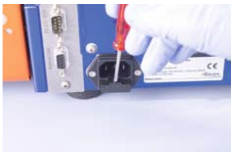
Figure 7.25: Removing the fuse holder.
