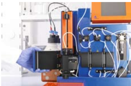
Figure 7.9: Removing the washing station.
