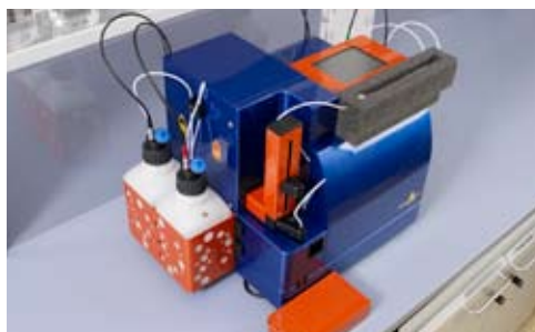
Figure 3.8: Close-up of the autoMACS Pro Separator - the needle arm and underside of the touch screen are supported by foam.
