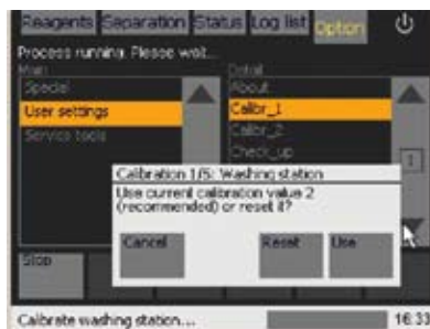
Figure 12.4: Calibration of the washing station. To use already saved settings select “Use”. To reset calibration settings (not recommended) select “Reset”.
