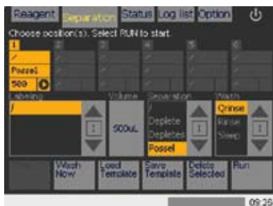
Figure 6.16: Performing MicroBead CD4 + cell separation with autolabeling (left) and without autolabeling (right). The cell separation (Possel) and wash conditions (Qrinse) for both processes are identical. Disabling autolabeling ("") influences the initial sample volume. For manual labeling it is recommended to dilute cells to a volume of 500 µL/10 8 total cells (refer to corresponding data sheet for further information).
