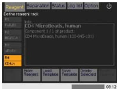
Figure 6.9: CD4 MicroBeads, human was assigned to reagent rack position R4, which was subsequently selected for deletion.
