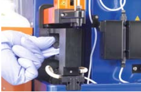
Figure 12.17: Unscrew the thumb screw.
