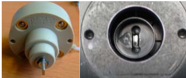
Figure 7.19: Inserting a new valve: take care to note the orientation of the valve.
