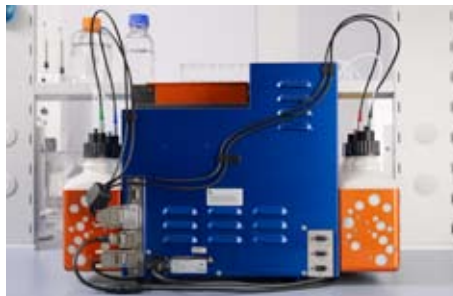
Figure 3.6: Sensor cables are attached to the back of the instrument as shown above.
