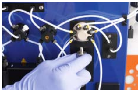
Figure 7.7: To remove the pump syringe the top screw must be turned anti-clockwise.
