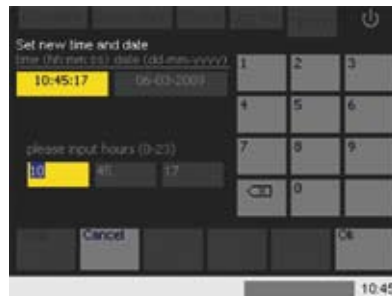
Figure 3.14: Select the desired field and use the numeric keypad to modify the date and/or time.
