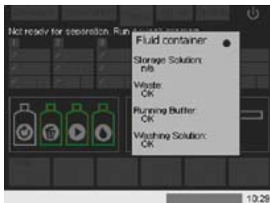
Figure 4.7: Fluid container status. By touching any fluid container symbol a popup box displays a text report of the fluid container status.
