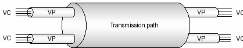
Fig. 3-1 – Data travel in ATM (from [26])
