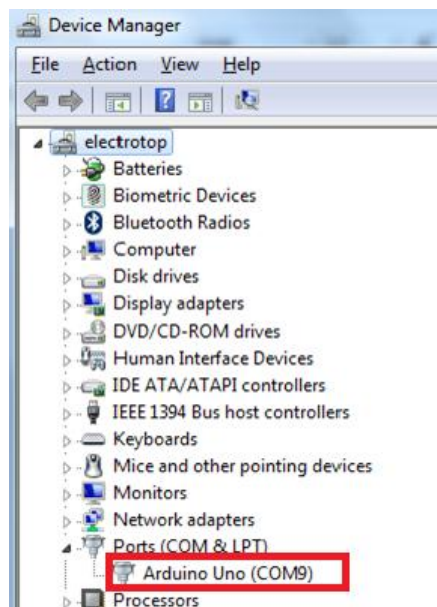
Fig. 3. A snapshot of Device Manager window, showing the number of serial (COM) port, to which the device is connected automatically.
