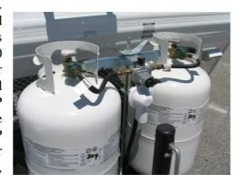
When there is a demand for gas from one of the appliances, the high pressure vapor is drawn from one cylinder, through the pressure regulator and reduced to the operating pressure of the appliance. The regulator allows the gas to be drawn from only one of the cylinders at a time. When the supply of gas from the tank is depleted,
