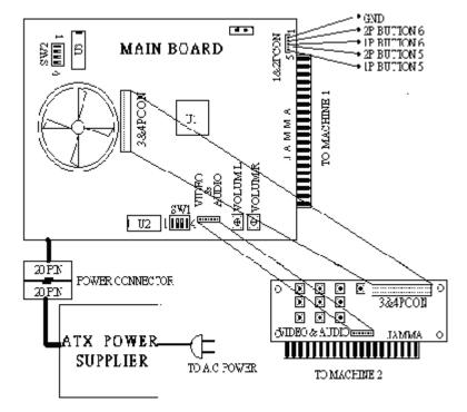
**Warning:** Use a wrong A.C. power input or connect the mainboard with JAMMA slot opposite direct would destroy power supplier or mainboard seriously.
