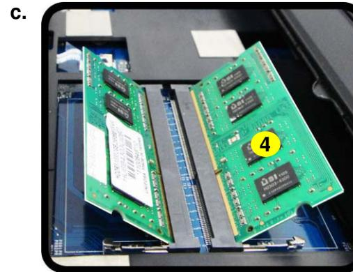
3. Gently pull the two **release latches** **2** & **3** **on the sides of the memory socket in the direction indicated by the arrows** ([Figure 8c](#)).
