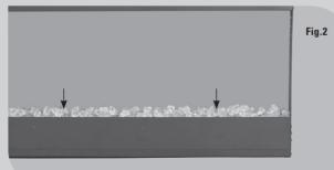
Put the front glass back and place the metal bracket on top of the glass so that the bracket secures it. Put the fasten screws back. Make sure the screws are tight and the glass is secured before continuing with the installation.
