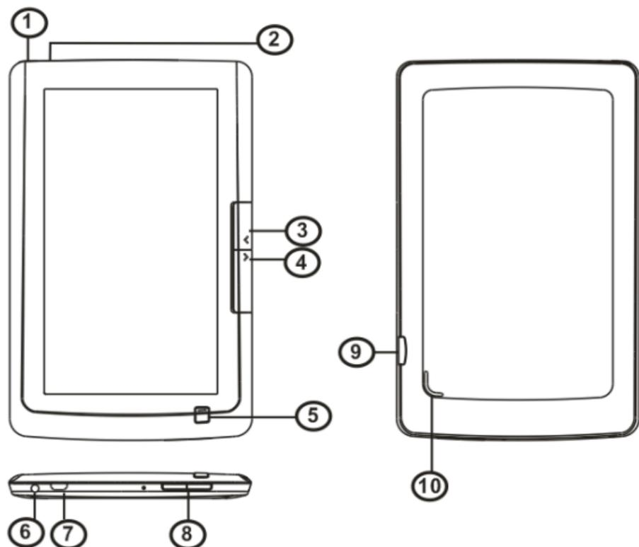
**1. Power button** – press and hold for 3 seconds to turn on/off. Press and hold for 6 seconds to restart.
