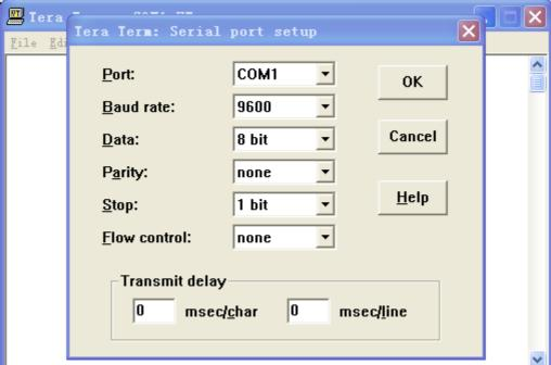
3. Connect ONU with relevant bunch port on the PC RS-232, then turn on the power, as following chart:
