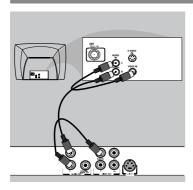
Use the composite video cable (yellow) to connect the DVD player's VIDEO(CVBS) jack to the video input jack(or the labeled as A/V in,Video In or Composite) on the TV(cable supplied). To hear the sound of this DVD player through your TV, use the audio cables(white/red)to connect AUDIO OUT(L/R)jacks of the DVD player to corresponding AUDIO IN jacks on the TV(cable supplied).
