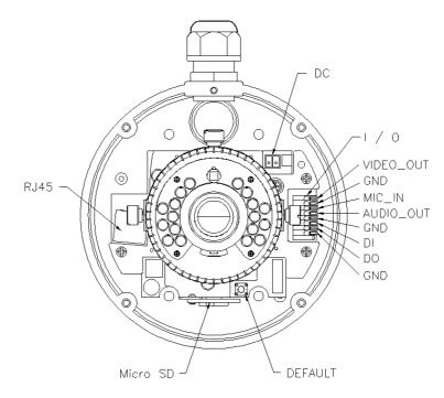
Connect power adaptor first, then connect the IP Camera to PC or network, and set up the network configurations according to the network environment. About I/O setting, please refer to chapter VII in User Manual: "I/ OConfiguration" for detail. The following picture shows a DC 12V connector for adapter jack plug.
