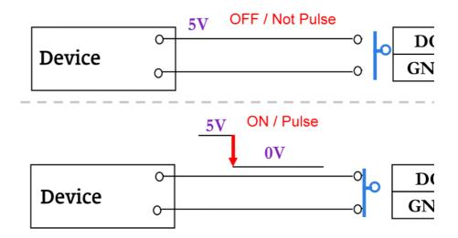
If you select "N.O" in "Input sensor setting", when external devise or circuit makes DI and GND pin connected, the camera input alarm is triggered, and then camera will execute the action user has set, for example, send snapshot to E-mail address.
