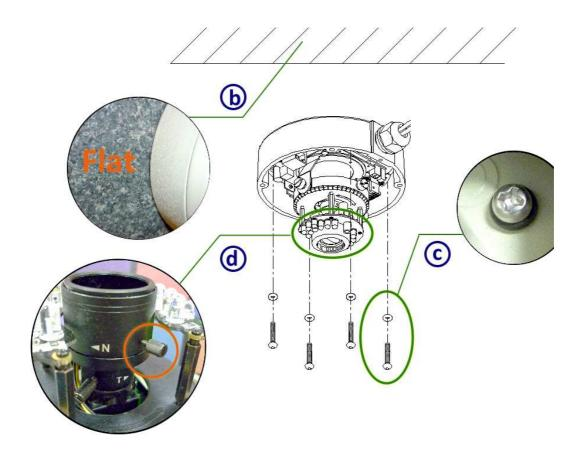
e. Use the 3-Axis bracket to adjust the camera to appropriate angle.
