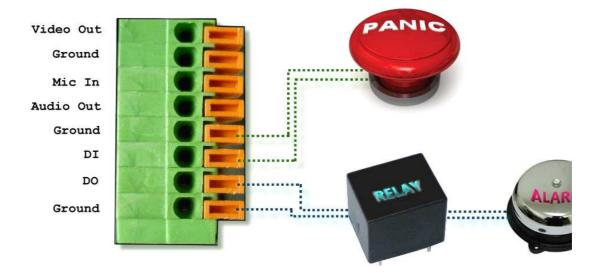
When no event happens, DO output is 5V (DO and GND are disconnected). When the camera detects event happening and triggers external alarm, DO output is 0V (DO and GND are connected).
