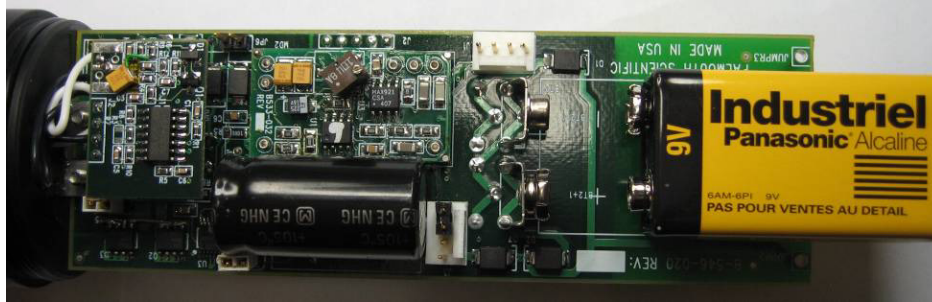
Figure 4-2 ATT-400 Battery Connections
