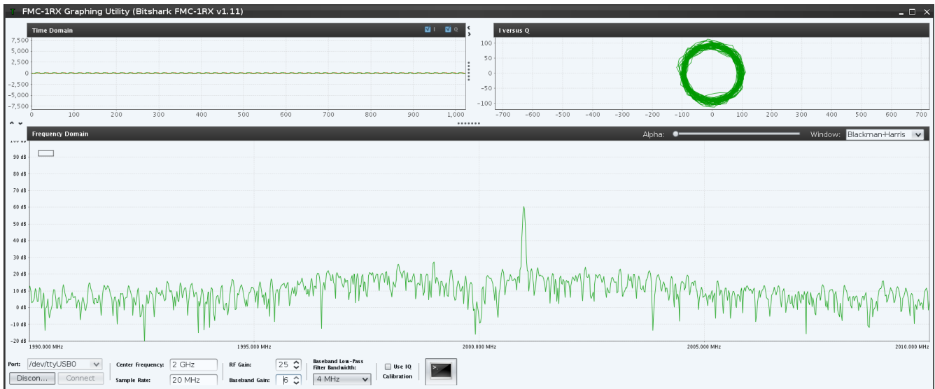
Figure 7: FMCGU screenshot showing an RF signal with the default configuration
