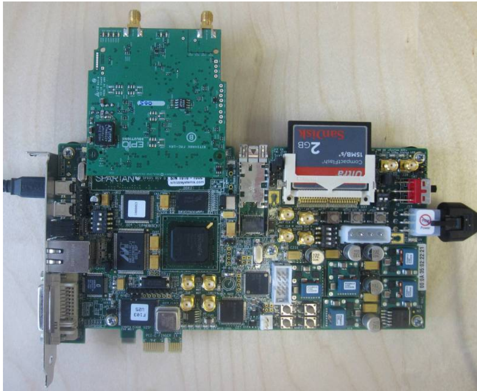
Figure 3: Xilinx SP605 with the FMC-1RX card inserted in the LPC slot
