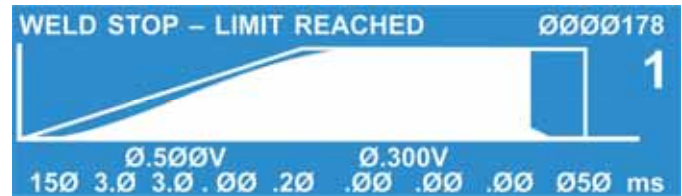
Weld to a Limit Waveform
