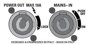
MAINS IN - Powercon® NAC3FCA power input connector (blue). To switch the amplifier on, insert the Powercon® connector and turn it in a clockwise direction into the ON position. To switch the amplifier off, pull back the switch on the connector and turn the connector in an anticlockwise direction into the POWER OFF position.
