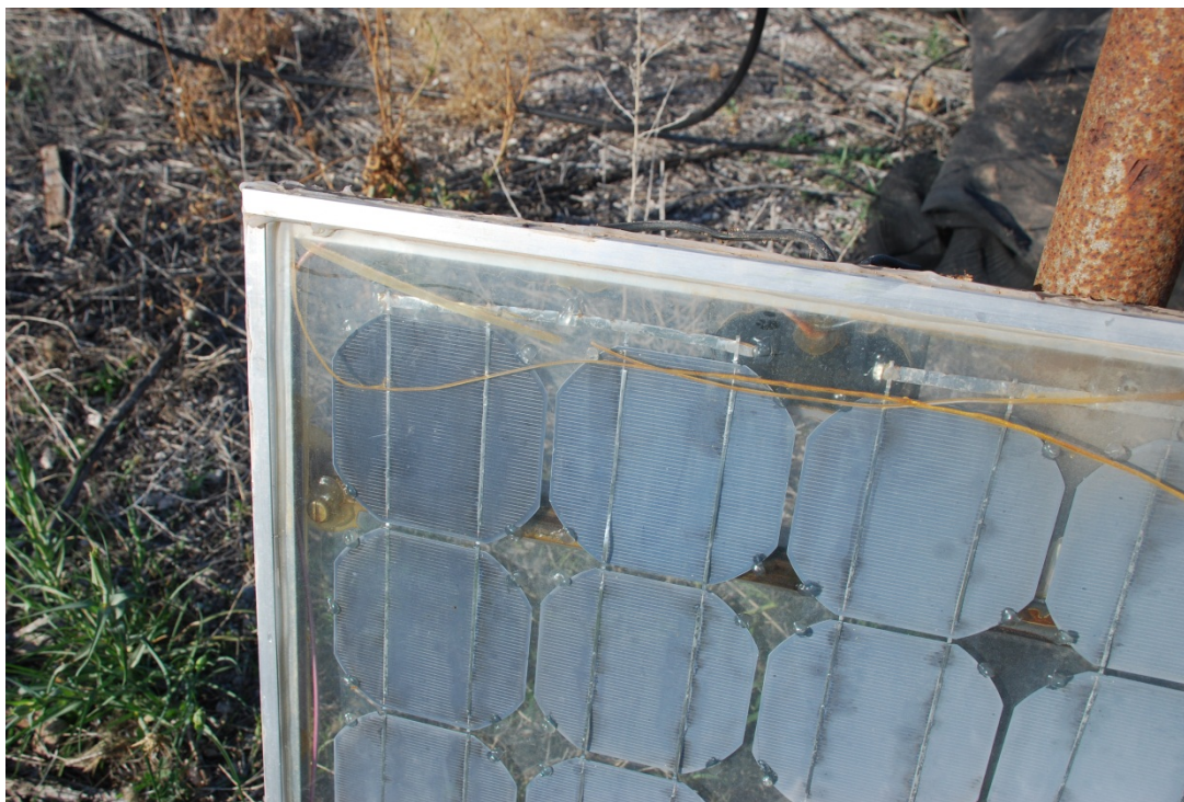
Glue separates from inside solar panel edges
