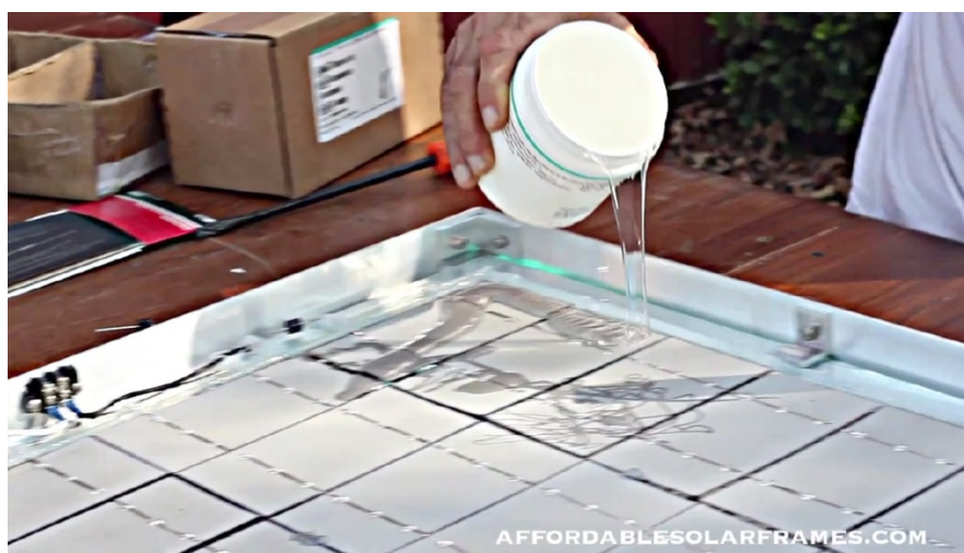
Pouring the Sylgard 184 Photo courtesy of affordablesolarframes.com/
