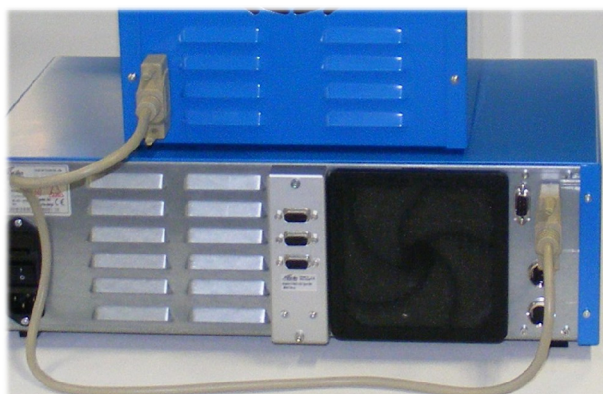
Fig. 6: Connecting the LED Cube 100 to the LED powerdrive
