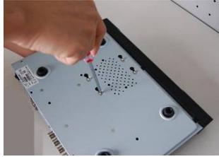
5. Fix the HDD firmly.
