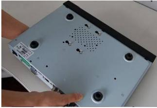
4. Turn the device upside down and then turn the screws in firmly.
