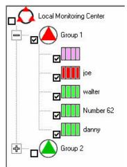
appear next to each group and each unit in the tree list. If a group's checkbox is checked, then all the units in that group will be polled. If any unit's checkbox is then unchecked, that unit will not be polled.
