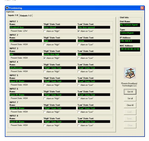
The provisioning window contains 2 tabbed views labeled "Inputs 1-8" and "Outputs 1-2". The default view is "Inputs 1-8". In this view, each of the ContactAgent's 8 digital input ports is represented by a 3-column line in the display. Each line consists of the following elements:
