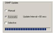
If the Automatic mode is selected, the Update button will not be displayed, and the countdown timer progress bar will indicate the time remaining until the next automatic poll begins. The polling interval as defined in the configuration file is also displayed.
