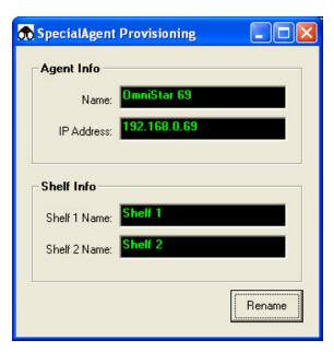
If the SpecialAgent type selected is capable of monitoring 2 shelves of equipment, then the user can assign a name for each shelf. After the desired shelf names are entered, pressing the "Rename" button will cause a password dialog to appear. If the correct password is entered, the new shelf names will be sent to the unit.
