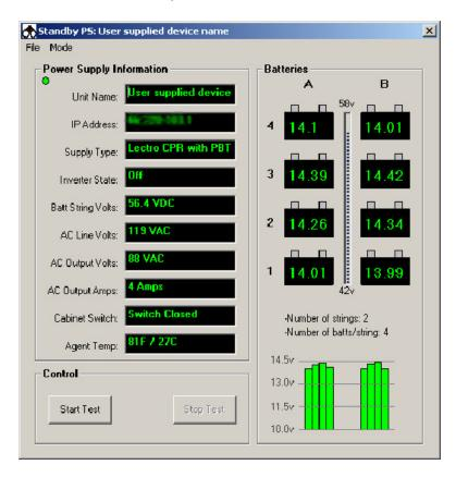
A graphical view of up to 4 batteries in 2 strings is displayed on the right side of the display window. Each battery's voltage is displayed within the corresponding battery graphic, and a vertical bar graph of the total string voltage is displayed in between the two battery strings. Under the right-side individual battery display, a bar graph displays the relative voltages of each of the batteries in the two strings.
