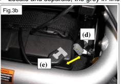
Battery Box, as shown in Figs.3a and 3b. Connect **Plug 1** Fig.1 of the Intermediate Cable, to **Socket** (**d**) Fig.3 and connect **Plug** (**e**) Fig.3 into **Socket 1** Fig.1.
