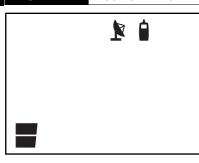
Your monitor is equiped with an optional "Out of range" indicator function, which will advise you when the two units are not communicating with each other. Out of range situations can be caused by distance or by physical interferences. **Range:** up to 250 meters/ 820 ft (open field); between 80 meters/ 262 ft and 100 meters/328 ft (indoors).
