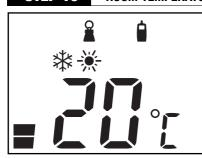
Your Angelcare@ monitor can also monitor your baby's room temperature and let you know when the temperature is to high or too low. A tripple BEEP will be heard if the temperature reaches levels out of the chosen range.
