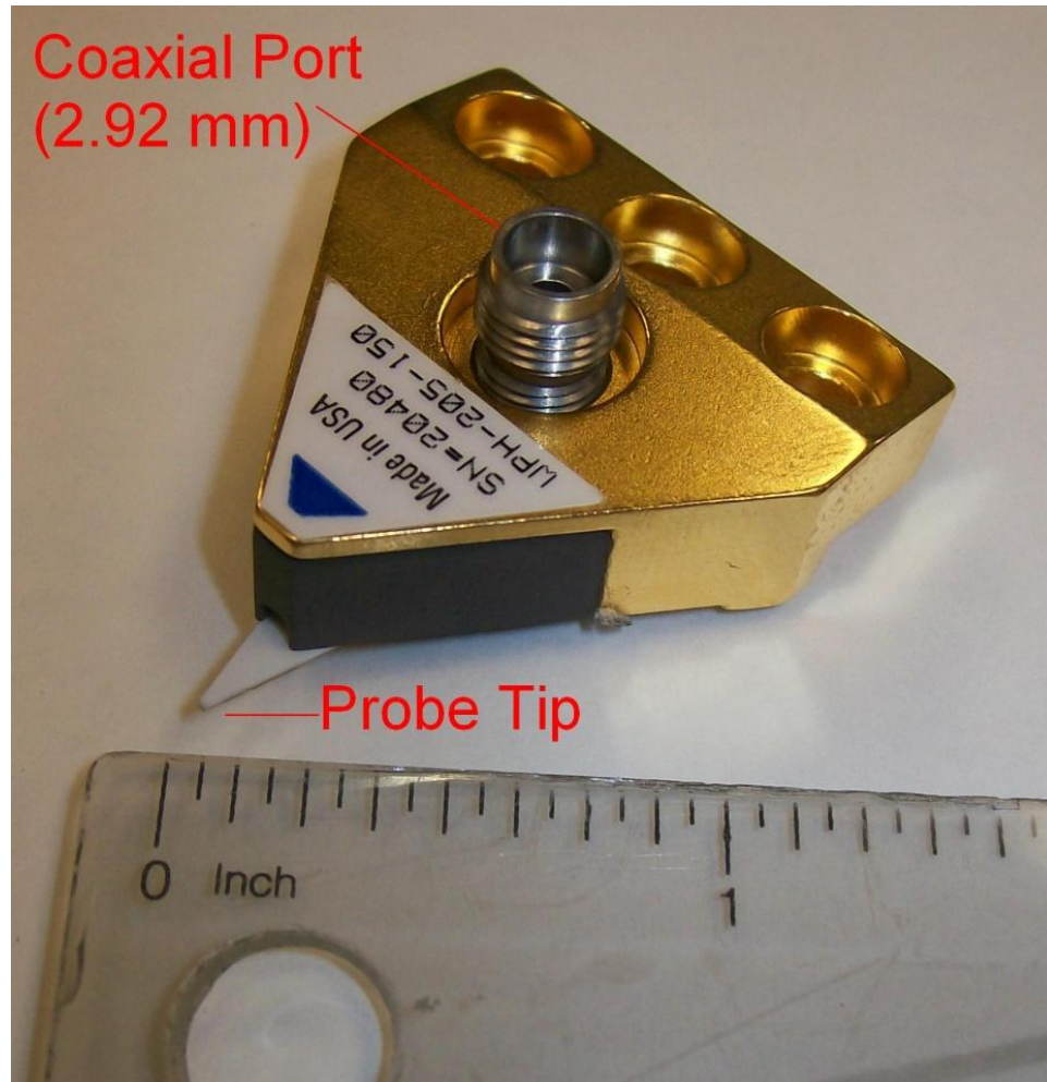
Figure 56 – Cascade Microtech WPH-205-150 Microprobe
