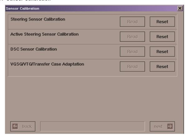
This set of functions allows sensors calibration. Some calibration procedures take several steps to complete – these are guided by wizard giving description for what should be done on each step:
