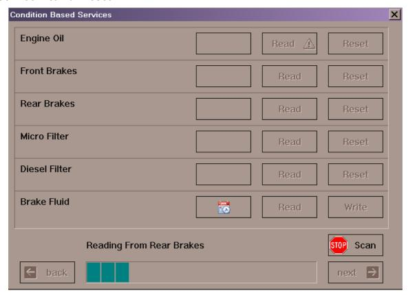
From this dialog you can check and reset the maintenance intervals. Some of the options are distance based, other are time based. Distance based intervals show how many kilometers remain until some action is needed (replacement or repair workshop visit). Time based intervals show at what date the action should be taken. There are options that have both time based and distance based values – whichever option expires first will trigger replacement event.
