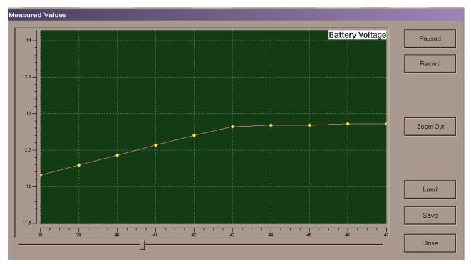
At this screen the data is refreshed at 50ms interval. When you push the "Playing" button, it will display graphically the change of the values, but will not record them. Click on "Record" to start collecting data which can be browsed back and forward with the scroll, saved in file (plain text file for easier offline analysis).
