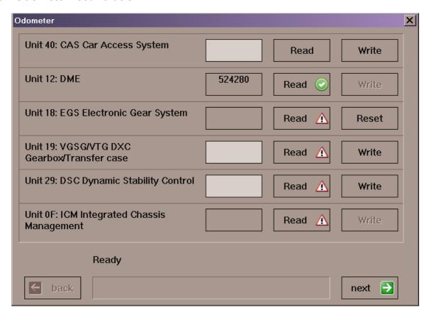
When you open the dialog, it starts automatic retrieval for some of the values. You can interrupt the scanning by pressing the "Stop" button (visible during scanning) and then click on "Read" for specific modules. Some units take more time to read their mileage and they are skipped during the auto scanning – you have to explicitly click "Read" for them.
