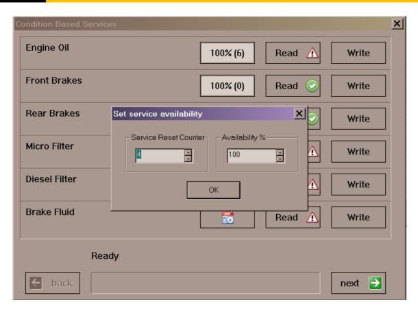
From the new dialog, you can change the counter of how many times the service has been reset as well as the current availability value. When you change the data, you have to click on "Write" to send the data to the unit.
