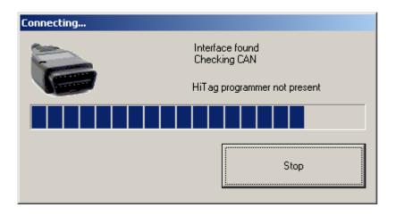
After successful detection of your interface, the software will check whether there is connected HITAG programmer and then will try to automatically detect body type of your vehicle.
