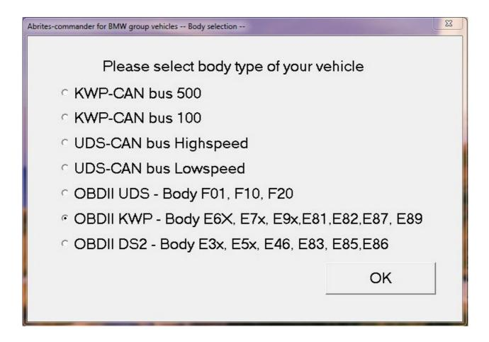
From this screen you should select type of the connection between your diagnostic interface and electronic control units in the vehicle. Connection types can be:
