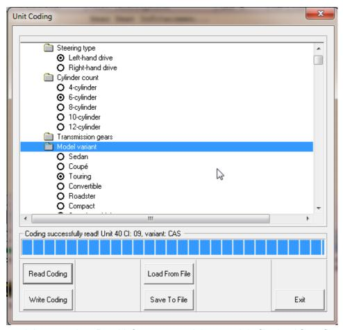
one module to another. Read it from one module, save it in file, load from file when the target unit is attached and write it in the device. From this dialog you can also restore coding from file backups, made by the central coding function.
