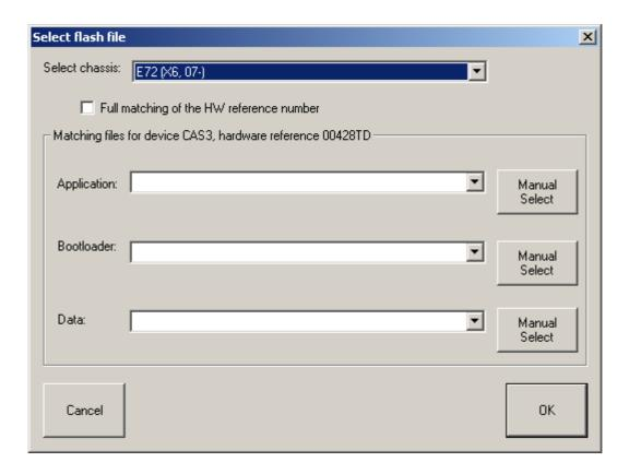
Before each reprogramming you will be asked about new data for UIF and ID stored in the unit. In some cases exchange data in UIF or ID is possible after reprogramming flash memory of the unit.
