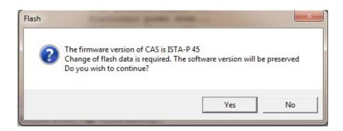
If you accept it, it will start a procedure that takes about 10 min. After it, the firmware version of the CAS3 will be the original one – no downgrade or upgrade is made. Once started, please do not interrupt the procedure.
