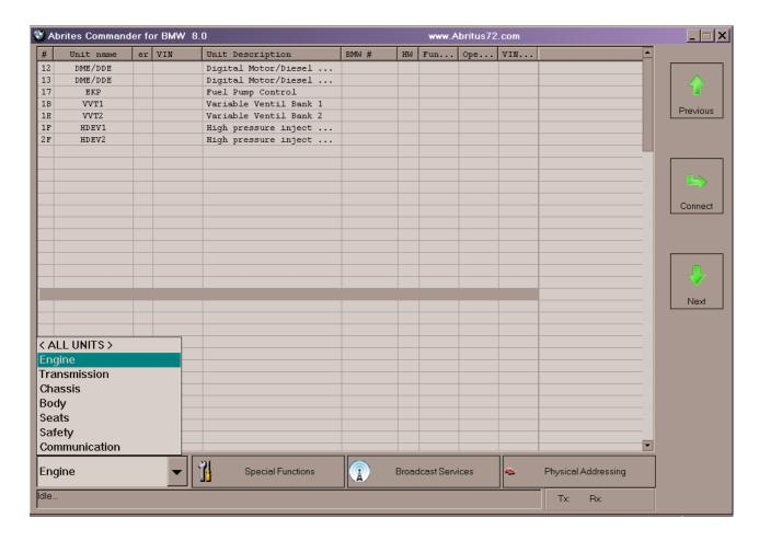
You can use the filter in the lower left portion of the screen to select which group of units is displayed. By default all units are displayed (in the example above we used filter to display just the units related to the engine).
