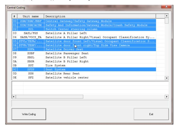
When you click on "Write Coding", the coding for all selected modules starts. You have a message area with status for each of the processing steps. Before changing the coding, each module data is automatically backed up in a file in windows temp directory. If needed, this file can be written back in the device with the unit coding function.
