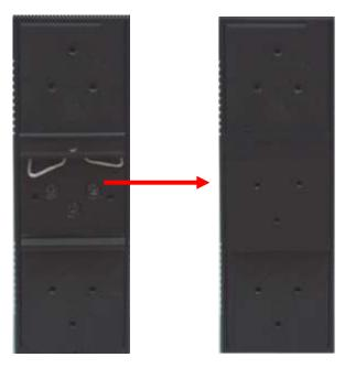
Step 2: Take the 6 screws that are included in the package and use them to attach the included wall mount to the switch as the picture shows below:
