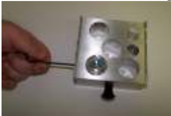
Figure 3: Fixing the sample in the Sample Stage.
