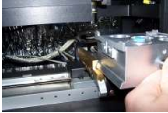
Figure 5: Slide the Sample Stage back into the dovetail rails.
