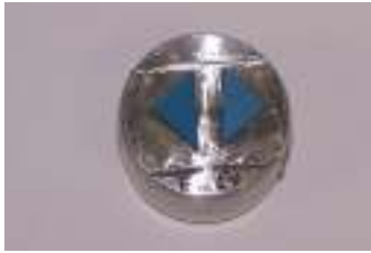
Figure 1: Sample mount. The sample is mounted to the glass slide with epoxy which and the glass slide is mounted to the puck using Crystal Bond.
