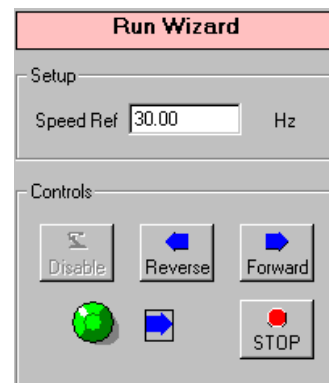
Figure 8.5a: Motor Running Forward
