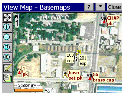
Good Control Point Geometry
