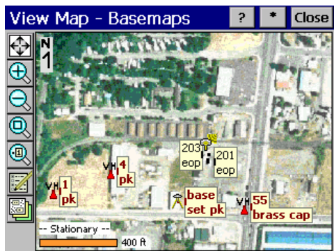
Poor Control Point Geometry
