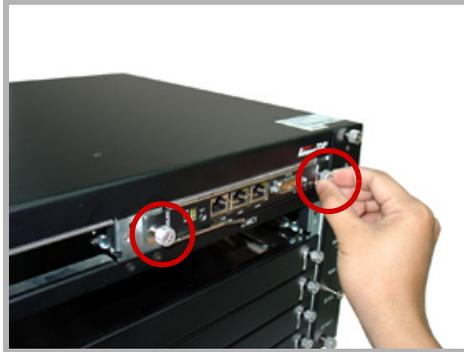
2. Pull the module handle outward until the card disengages from the chassis.
