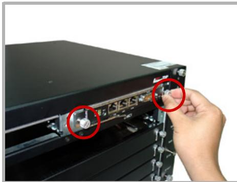
The aCMM-2000 powers up instantly and the ACT LED lights up green. When two aCMM-2000 modules are installed, the ACT LED of the backup module blinks.
