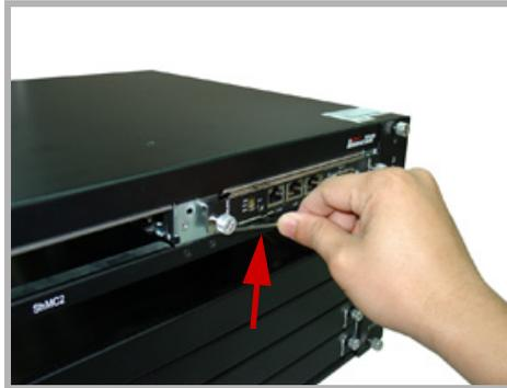
6. Tighten the retention screws on both sides of the module to secure.
