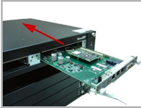
4. Push the module to the slot until the metal tacks are inserted into the chassis holes.
