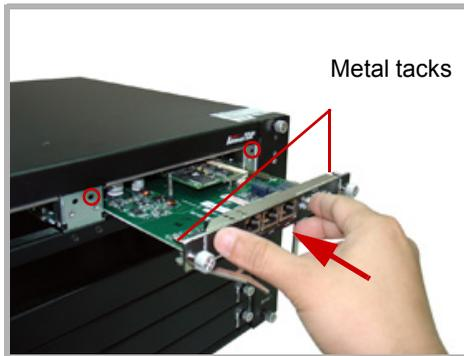
5. Push the handle inward to set the module in place.
