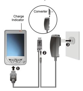
3. The charge indicator glows amber when charging is in progress. Do not disconnect your Pocket PC from AC power until the battery is fully charged, as indicated by the amber indicator turning into green. This will take a couple of hours.
