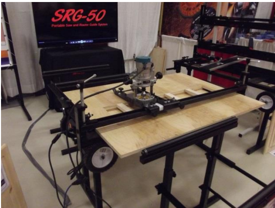
Set up with router in sled
