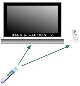
An iPod docking station connected to a B&O TV. A single push on the Beo4's DVD button will turn on the TV, open a Scart input, turn on the iPod dock and shift to operate the iPod.
