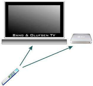
An Apple TV connected to a B&O TV. A single push on the Beo4's DVD button will turn on the TV, open a HDMI input, turn on the iPod dock and finally shift to operate the Apple TV.
