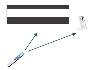
An iPod docking station connected to a B&O audiomaster. A single push on the Beo4's CD button will turn on the audiomaster, open the A.TAPE input, turn on the iPod dock and shift Beo4 to operate the iPod.
