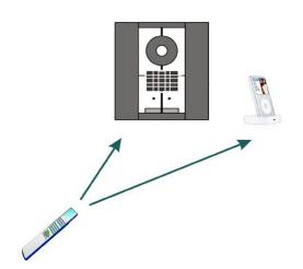
An iPod docking station connected to a B&O audiomaster. A single push on the Beo4's AMEM / A.TAPE button will turn on the audiomaster, open the AAUX input, turn on the iPod dock and shift Beo4 to operate the iPod.
