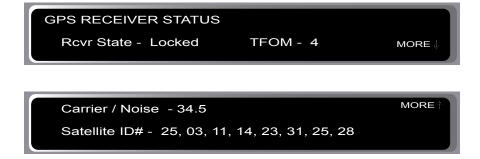
Receiver State: This shows the current state of the GPS receiver subsystem. The state may be: acquire, locking, or locked. When locked, the GPS receiver is synchronized to the signal and it is disciplining the internal oscillator to remove frequency and time errors.
