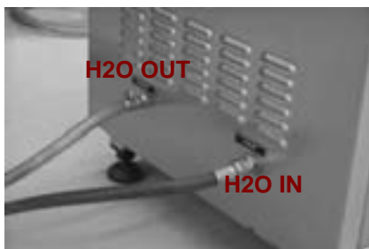
Fig. I-4a cooling water inlets and outlets.
