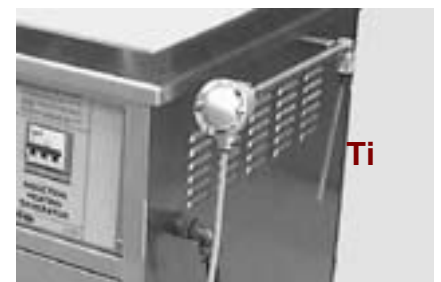
Fig. I-4c detail of the immersion thermocouple
