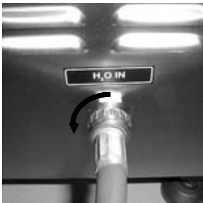
Fig. IV-2a Detail of the water inlet fitting
