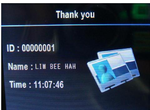
Also, the punching record will be saved into the machine flash. Besides, a door lock signal will be released for opening door.
