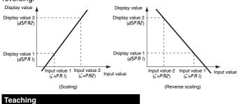
Settings for scaling can be made using the present measurement values instead of inputting values with the SHIFT and UP Keys. This is a convenient function for making settings while monitoring the operating status, for calculating amounts by tare reduction (to measure only the contents), or when the result should be zero but the display is not zero for some reason.
