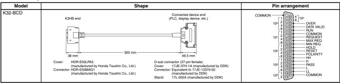
Note: The BCD Output Cable has a D-sub plug. Cover: 17JE-37H-1A (manufactured by DDK); Connector: equivalent to 17JE-23370-02 (D1) (manufactured by DDK)
