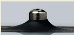
Droplet "flattens out" on unconditioned pedestal
