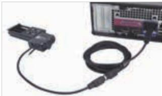
T-Series devices can connect to a computer's serial port with a T-DSUB9 adaptor and a T-DC06 cable.
