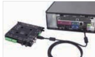
Stand-alone controllers also have the option to connect directly to a computer's USB port with a U-DC06† cable.
