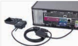
T-Series devices can connect to a computer's USB port with a T-USBDC\* cable.
