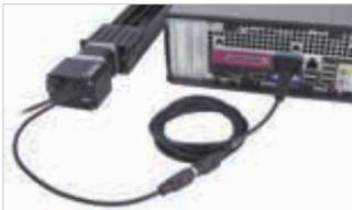
A-Series devices can connect to a computer's serial port with a T-DSUB9 adaptor and a T-DC06 cable.
