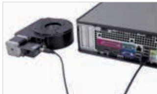
X-Series devices can connect to a computer's USB port with a X-USBDC\* cable.
