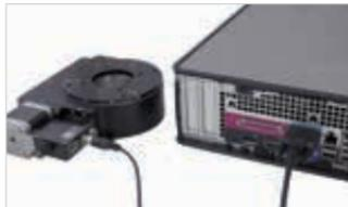
X-Series devices can connect to a computer's serial port with a X-SDC cable.
