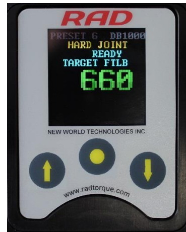
Figure 3.3.2-2: Main Screen – Hard Joint Mode
