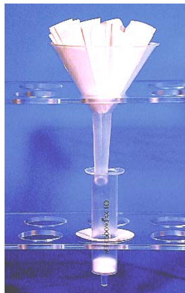
Figure 2: Correct use of the folded filters
