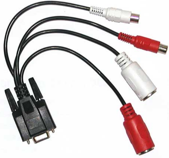
Firebox rear view (top) plus breakout cable, which connects MIDI and S/PDIF I/O.
