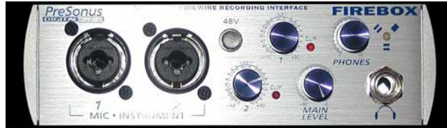
Firebox front panel, sporting Neutrik plugs, independent gain controls for the two preamps, 48V Phantom power, main level adjustment and headphone jack and level control.
